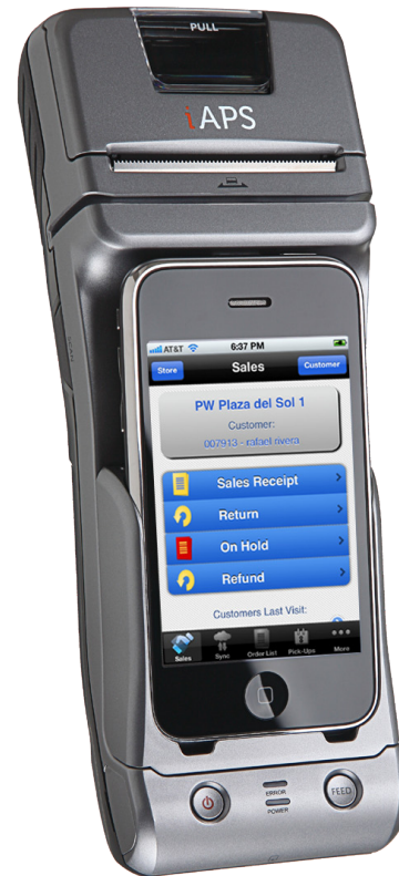
The iAPS sled adds scanning, secure card swiping, and receipt printing to the iPhone.
